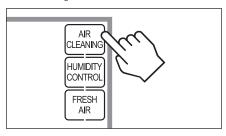
If installed, air cleaning can operate in five different modes. Air cleaning will activate the fan for the purpose of air cleaning.
