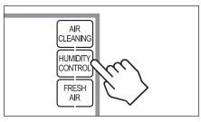
The Humidity Control screen can be used to control both humidification and dehumidification.
