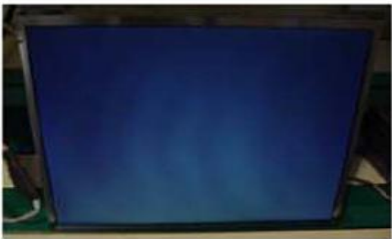
Panel Mura, Light leakage
