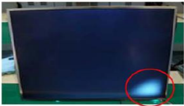
Panel Mura, Light leakage
