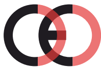
False CE Mark (too close)
