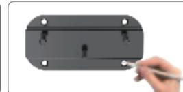
Step 2: Place the wall fixing sheet metal onto the wall/ceiling and draw 4 marks aligning the four hole positions.
