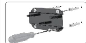
Step 3: Drill holes at marked locations, insert anchors into the holes, and then insert the screws through the wall fixing sheet metal and rotate the mounting into the anchors.
