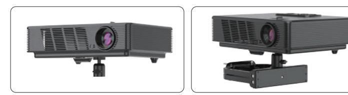
(1) Take out the ball head and attach the projector to the ball head first.
