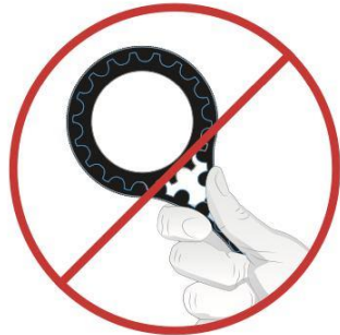
DO NOT USE BELT AS A SPROCKET REMOVAL TOOL
