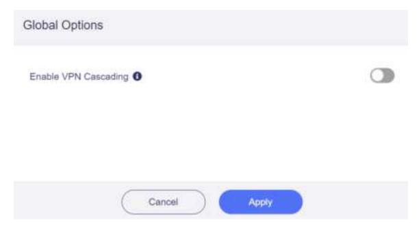
VPN Cascading, If this option is enabled, when you have both VPN server and VPN Client running on this router, clients connected to the VPN server will further be routed to the VPN client tunnel. Learn more about VPN Cascading.
