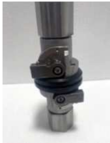
2. Push the parts together so the pins are compressed.
