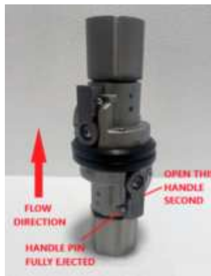
5. Compress the handle pin and twist it to open the 2nd valve. The pin on the handle will fully eject when the valve is completely open. If there is pressure in the system, the coupling that the flow will reach first should be opened last.
