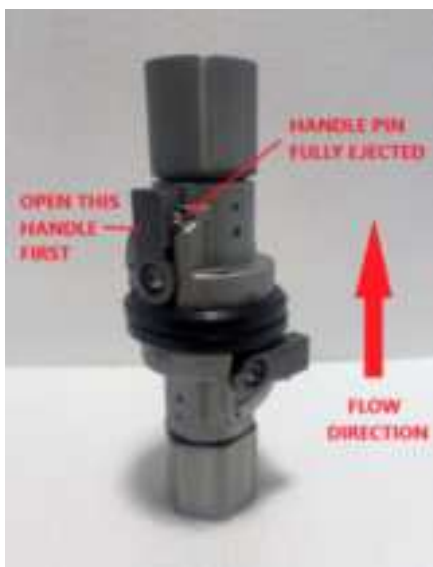
4. Compress the handle pin and twist it to open the 1st valve. The pin on the handle will fully eject when the valve is completely open. If there is pressure in the system, the coupling that the flow will reach last should be opened first.
