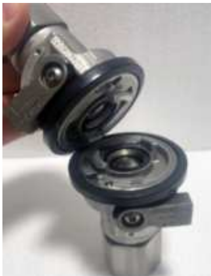
1. Align the lugs with the grooves on the mating coupling.
