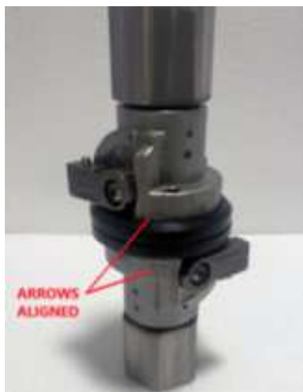
3. While continuing to push the parts together, twist the two couplings until the arrows align. The parts will "click" when fully engaged.
