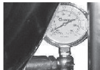
Each day confirm the jacket water level by checking the water gauge.
