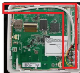
Example Proper Shape of the Bent Cable
