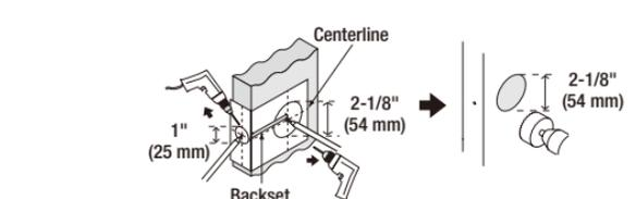
**2** Prepare the door jamb – use the strike plate as a template to drill the latch and screw holes and chisel out the mortise. The strike plate must fit flush with the surface of the door jamb.
