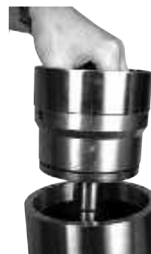
16. Remove cylinder barrel.
