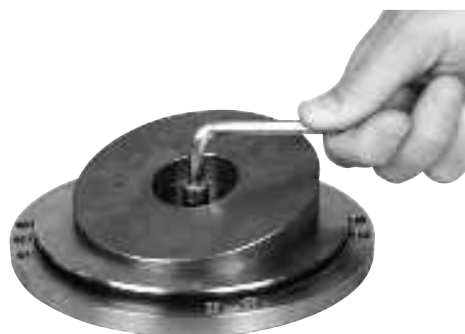
28. Loosen and remove screw from swash plate.
