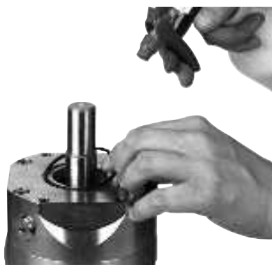
33. Spray with water and mount O-ring.
