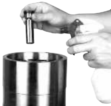
21. Spray with water and mount pistons.
