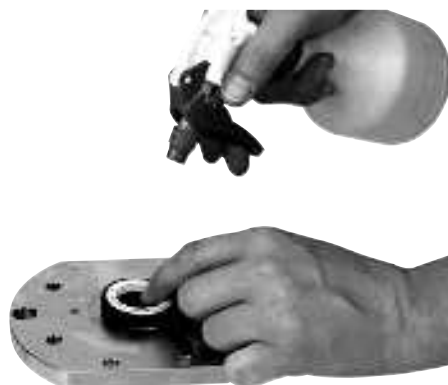
34. Spray shaft sealing with water before mounting.
