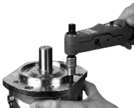
43. Tighten screws to 30Nm.
