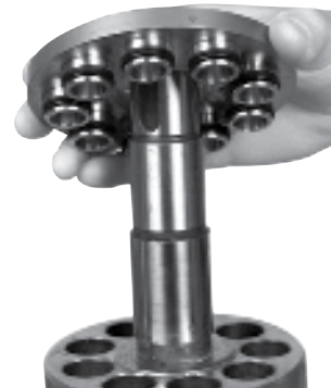
24. Remove thrust plate.
