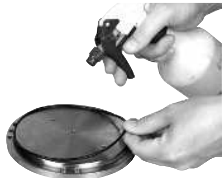
22. Spray with water and mount O-ring on end cover.
