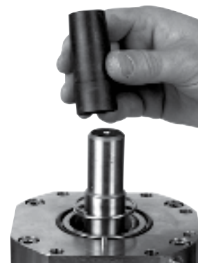
38. Mount special tool on shaft.
