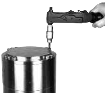
31. Tighten 10 screws to 30Nm.
