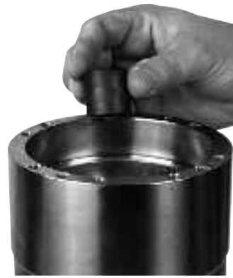
18. Mount retainer on top of the spring.
