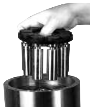
12. Remove pistons and retainer plate.
