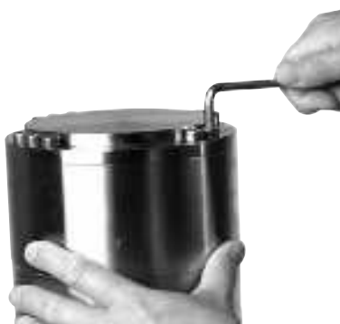
9. Loosen and remove 10 screws.
