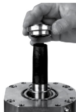
40. Mount sealing (smallest diameter pointing down).
