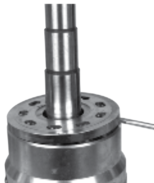
23. Loosen thrust plate from cylinder barrel.
