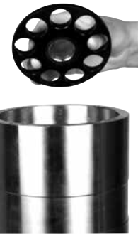
20. Place retainer plate on top of retainer ball.
