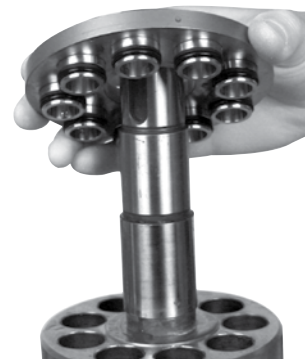
24. Remove thrust plate.
