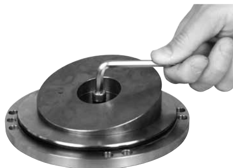
28. Loosen and remove screw from swash plate.
