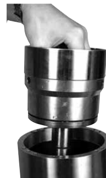
16. Remove cylinder barrel.
