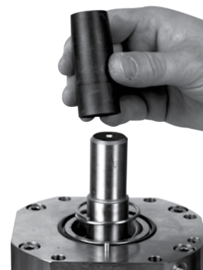
38. Mount special tool on shaft.
