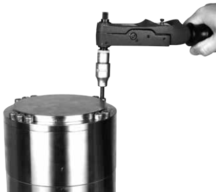
31. Tighten 10 screws to 30Nm.
