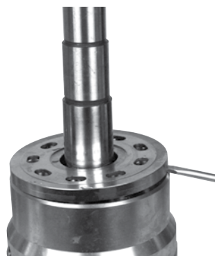
23. Loosen thrust plate from cylinder barrel.
