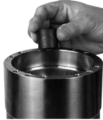
18. Mount retainer on top of the spring.
