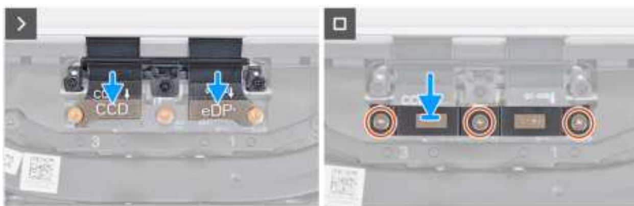
Figure 52. Installing the system board
