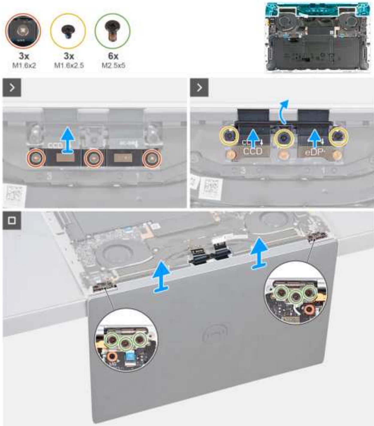
Figure 42. Removing the display assembly
