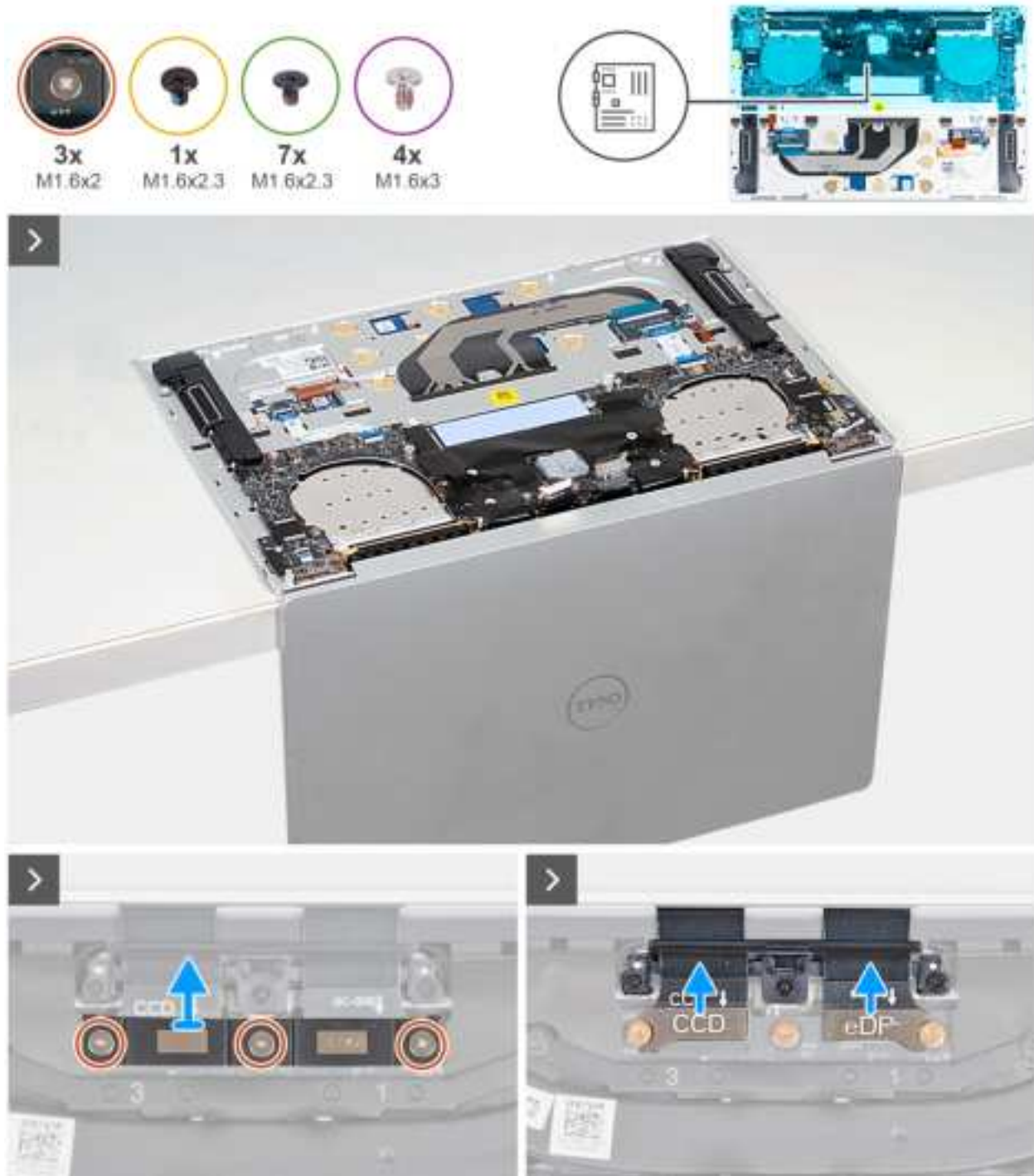
Figure 46. Removing the system board
