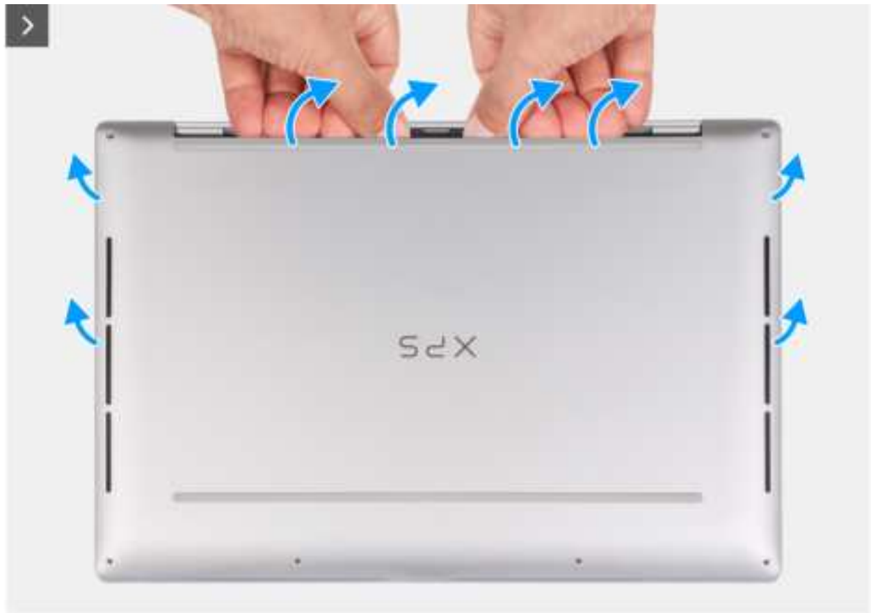
Figure 11. Removing the base cover
