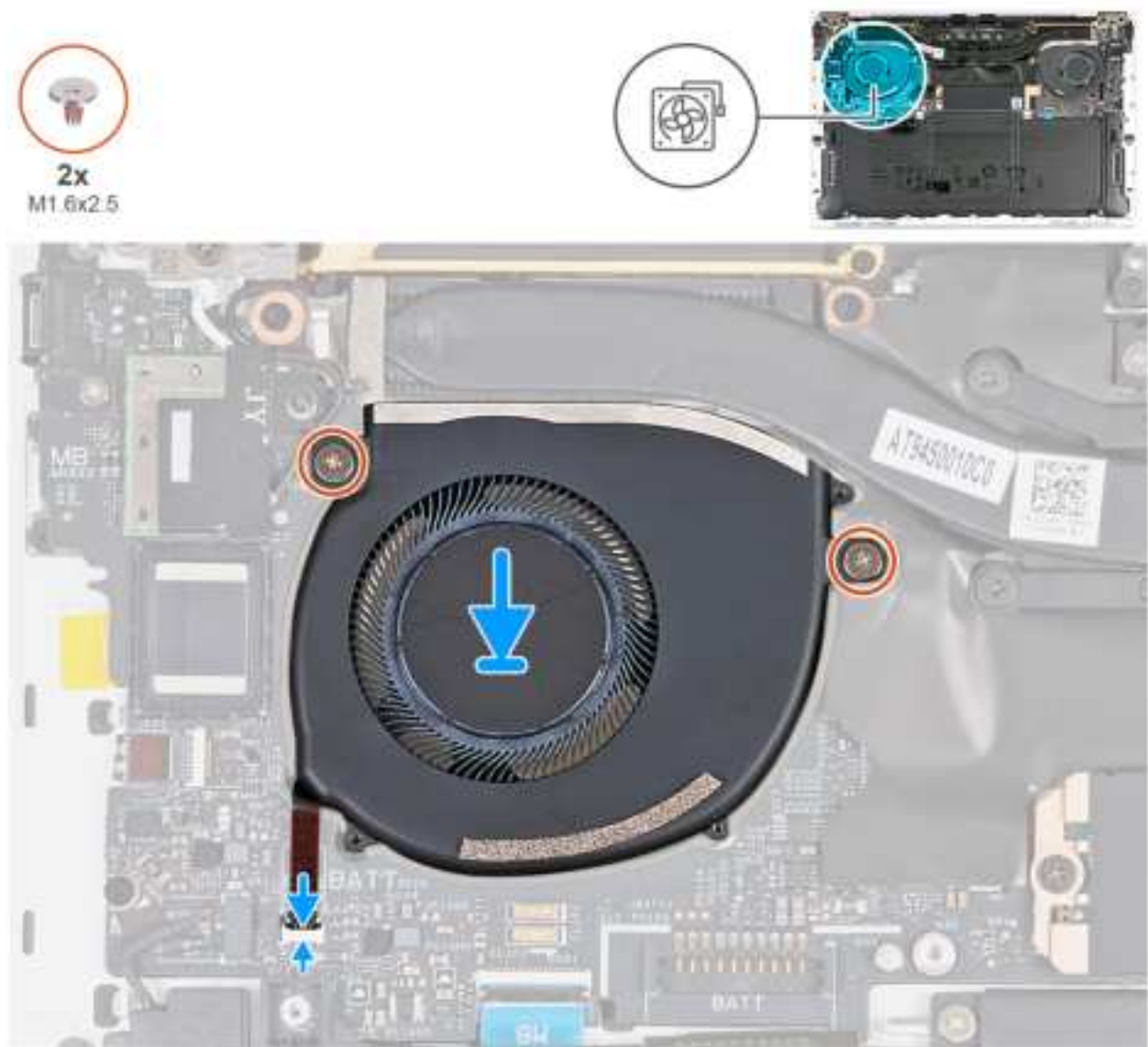
Figure 39. Installing the right/video fan
