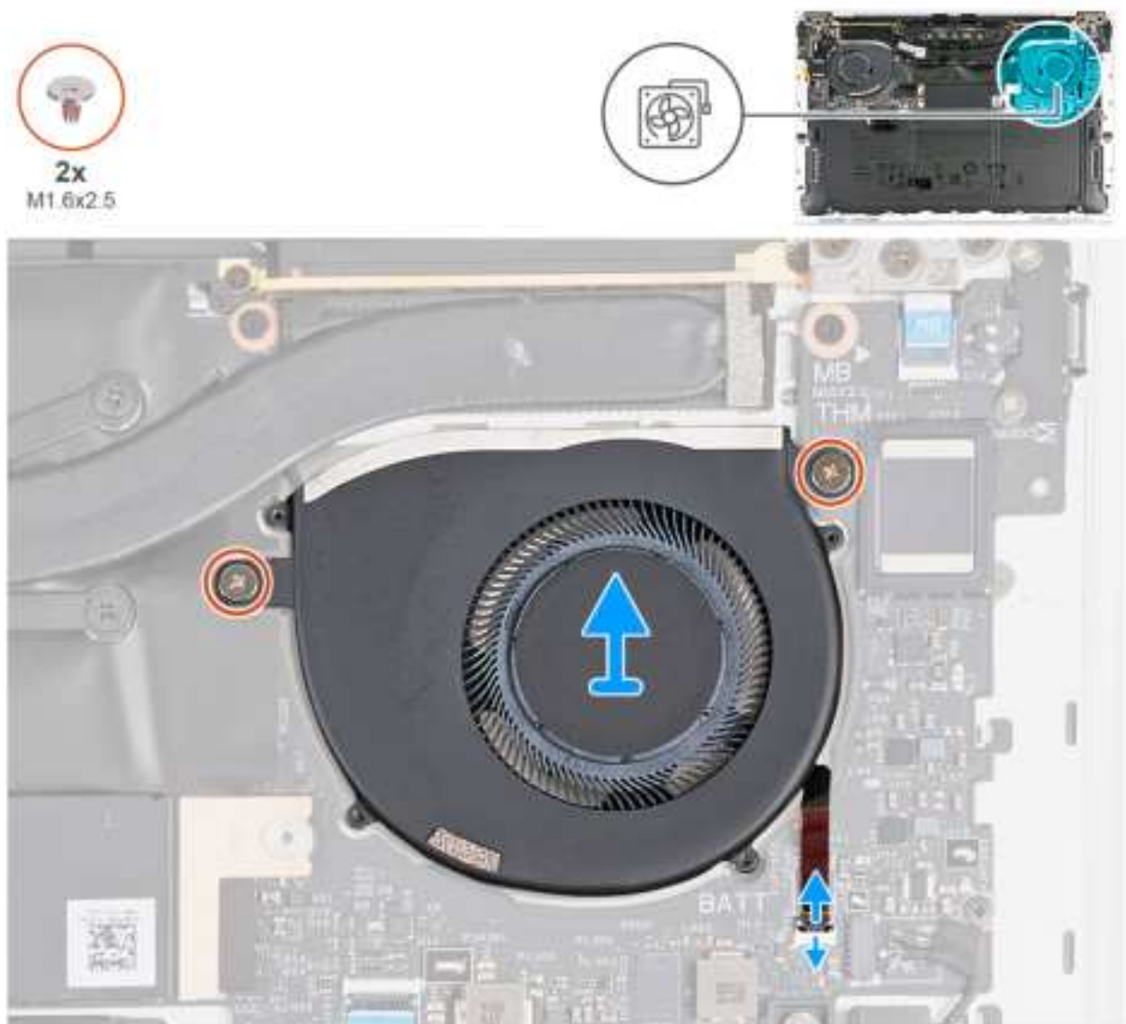
Figure 36. Removing the left/processor fan
