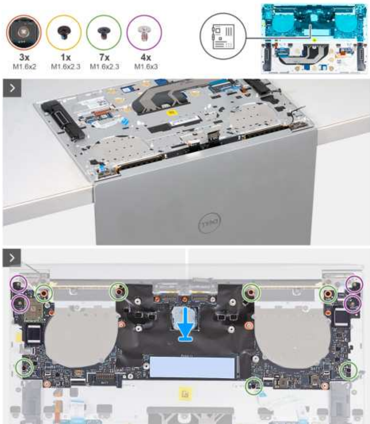
Figure 50. Installing the system board
