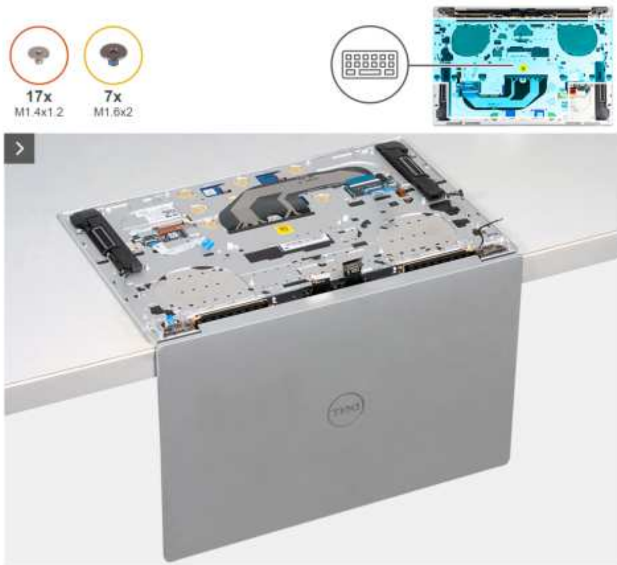
Figure 55. Removing the keyboard
