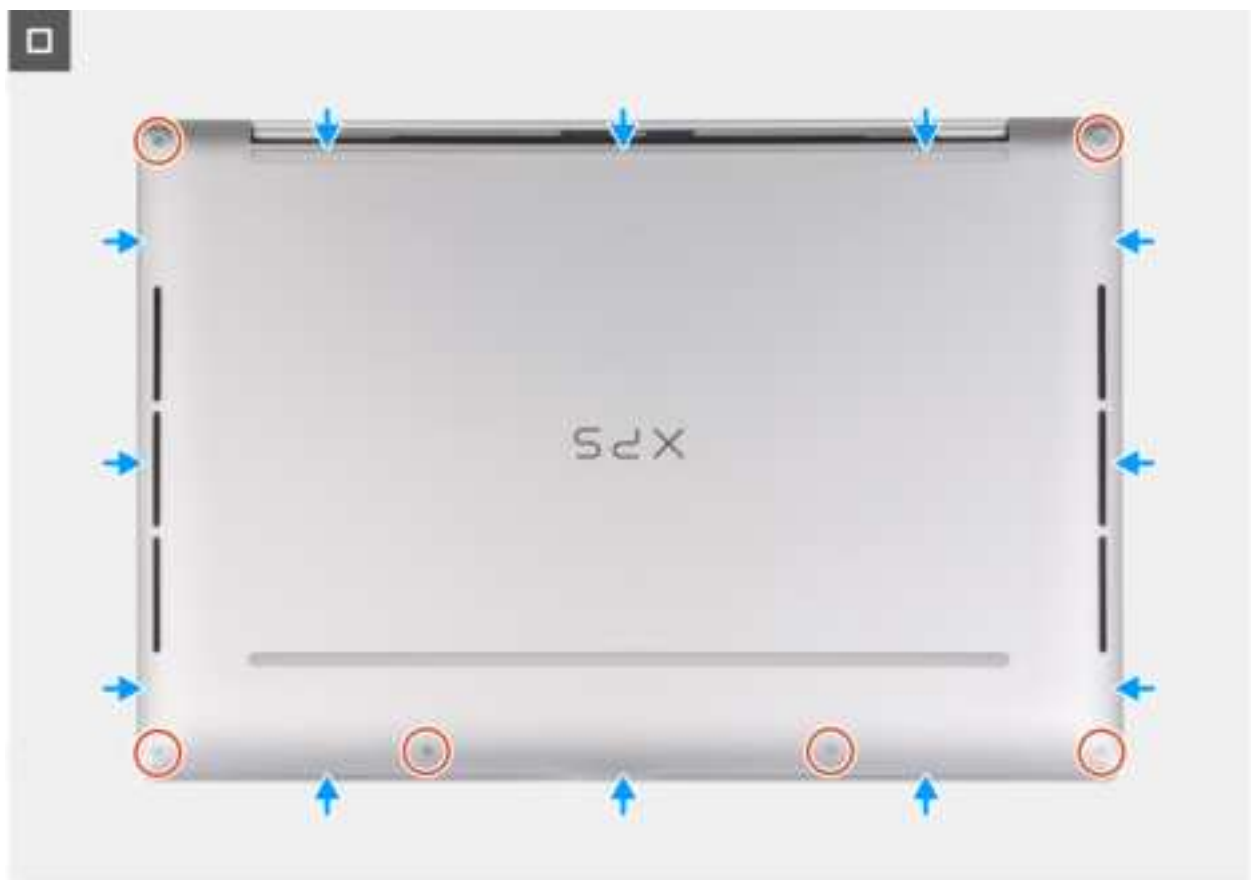
Figure 16. Installing the base cover
