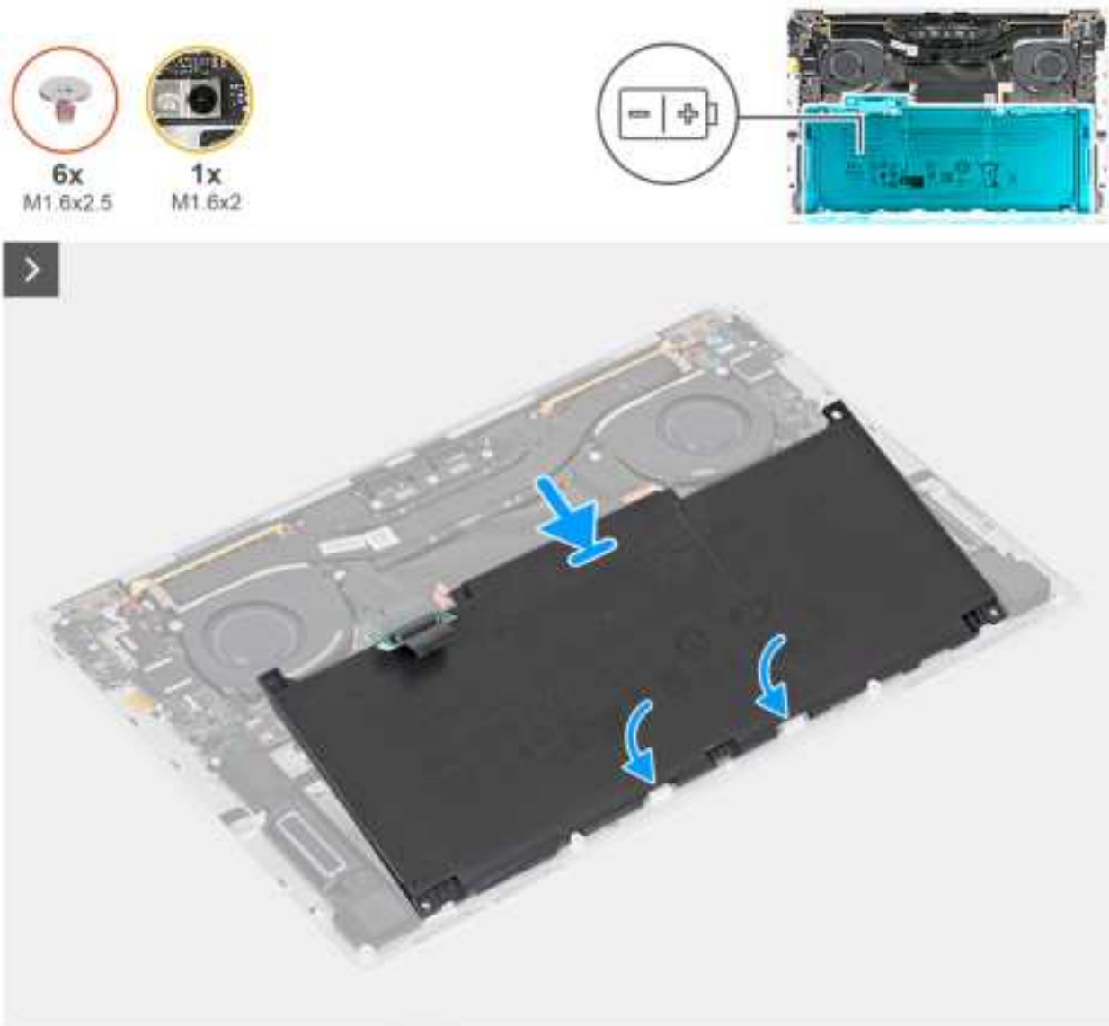
Figure 22. Installing the battery
