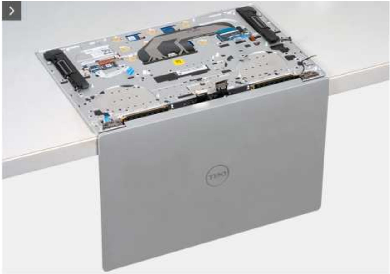
Figure 59. Installing the keyboard
