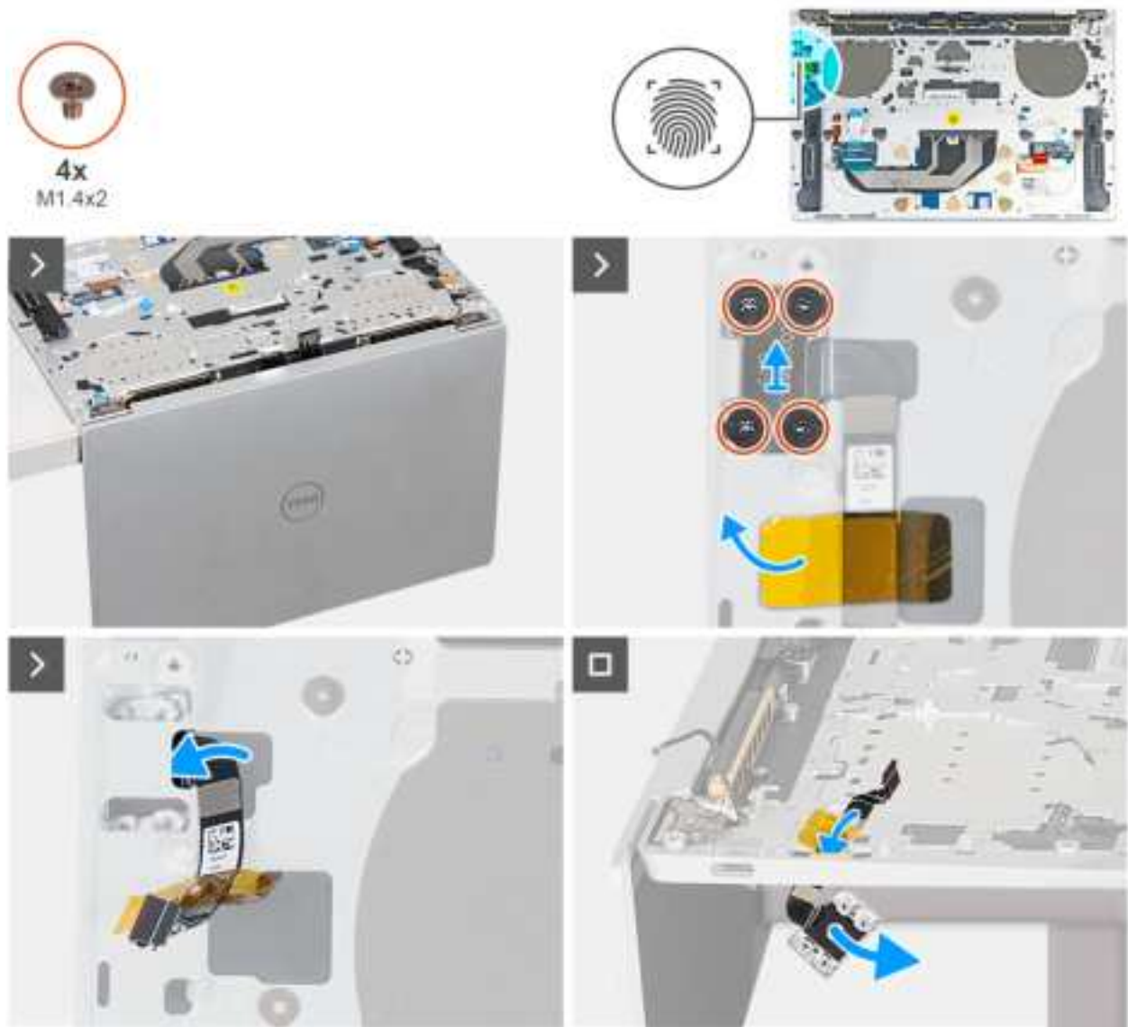
Figure 53. Removing the power button with fingerprint reader
