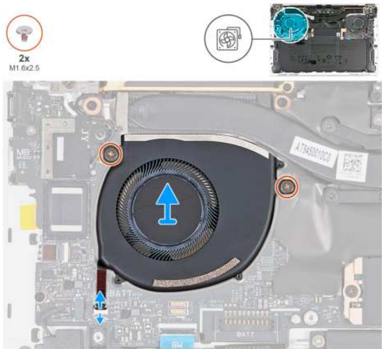
Figure 37. Removing the right/video fan
