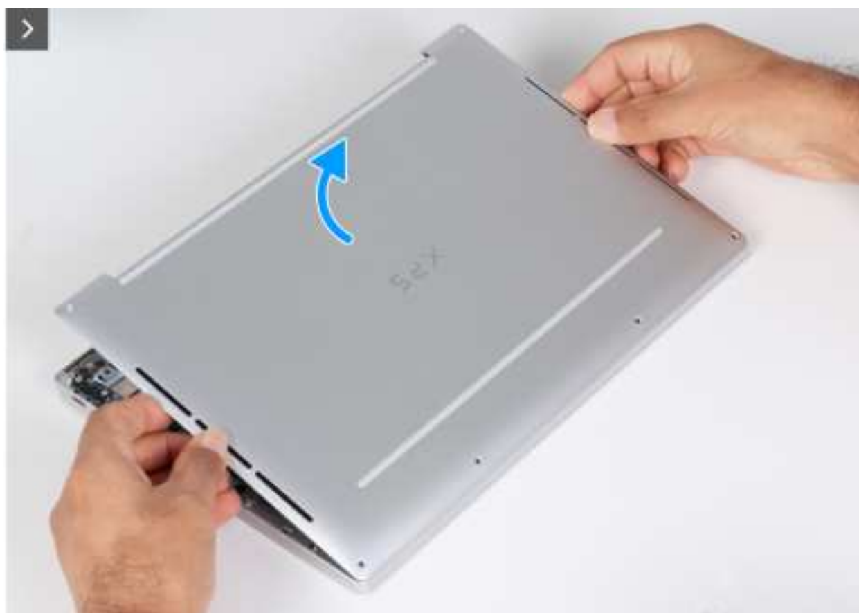
Figure 12. Removing the base cover
