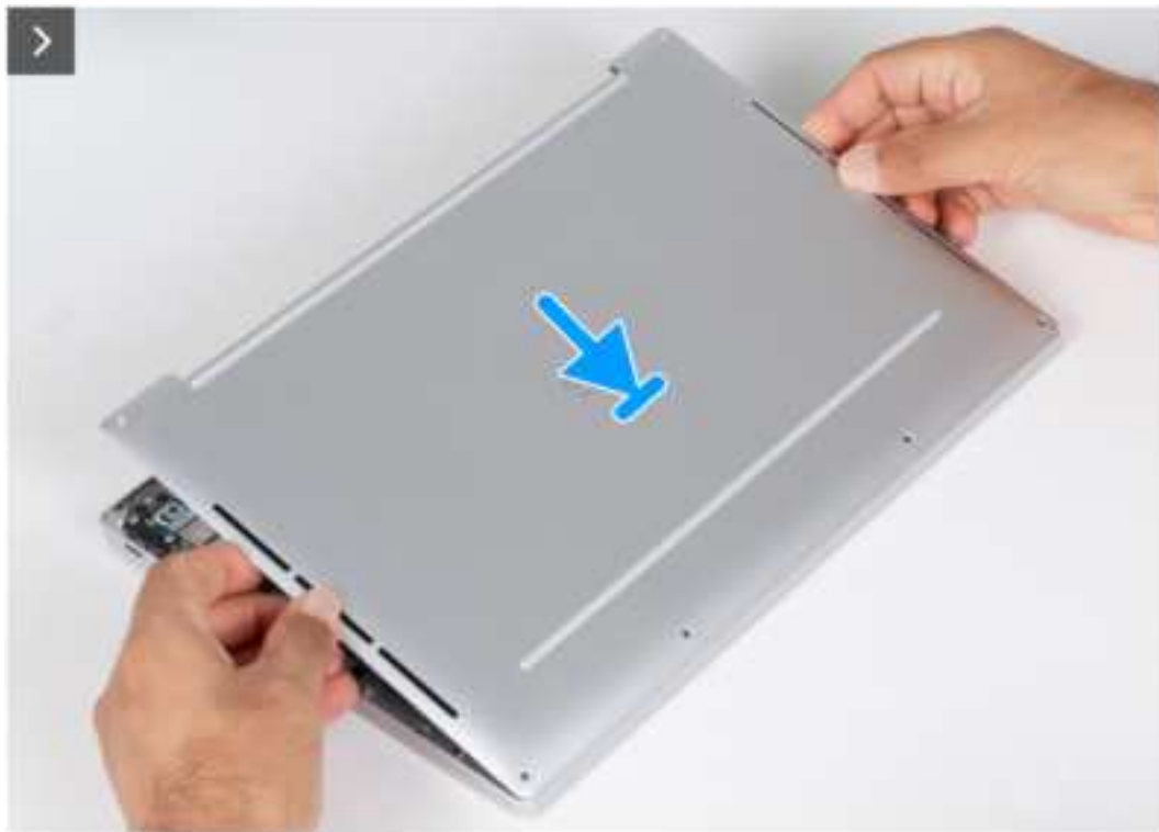
Figure 15. Installing the base cover
