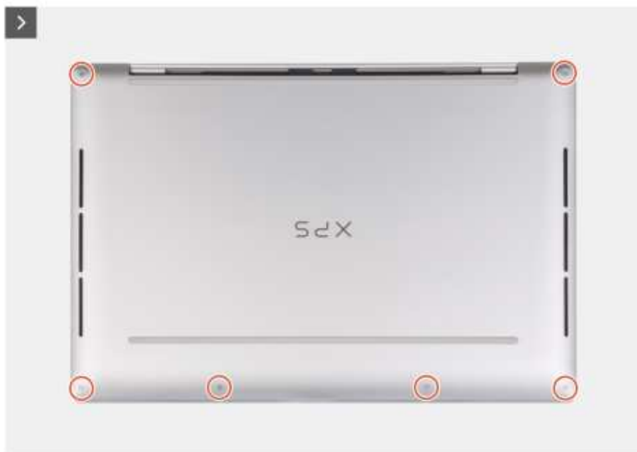
Figure 10. Removing the base cover
