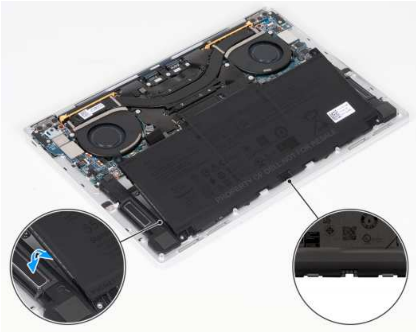
Figure 21. Lift the battery at an angle less than 30 degrees
