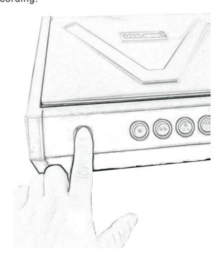
(2) Directly record the password and enter it (If the length of password is less than 6 digits, you need to wait for 6 seconds to confirm each time; if the length of password is equal to 6 digits, it will be automatically confirmed without waiting). After successful entry and confirmation, it will sound once and flash for 3 times. You need to enter passwords for 2 times. There will be a long beep after successful recording.
