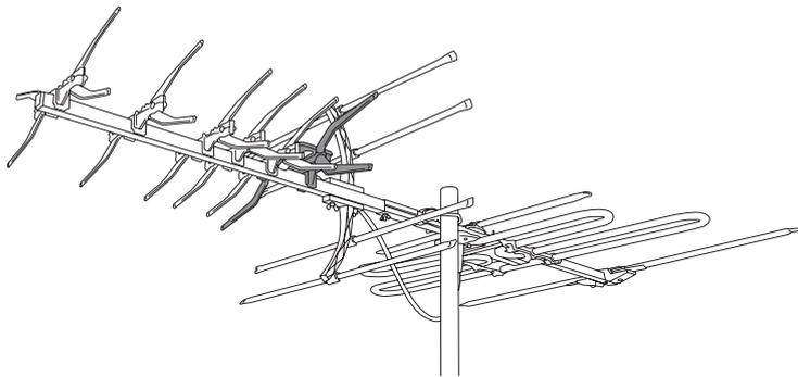
2) Click in the X type balun to the sixth mould located on the front 609mm boom. Ensure the connection points on the X type balun face the back of the antenna.
