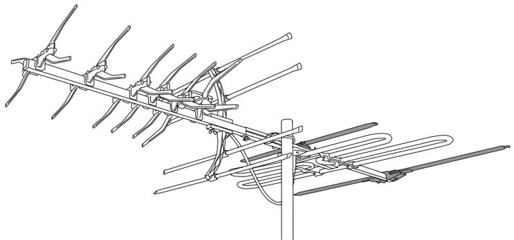
4) Snap out the three riveted swivel lock elements on the back 714mm boom.
