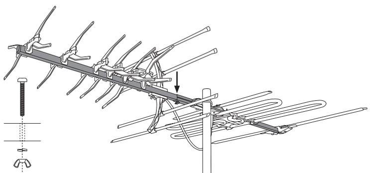
6) Join the front 609mm boom to the back 714mm boom using the 3/16" Philips head bolt, spring washer and wingnut provided in the small plastic bag. Make sure you install the spring washer and wingnut on the underbody of the boom body.
