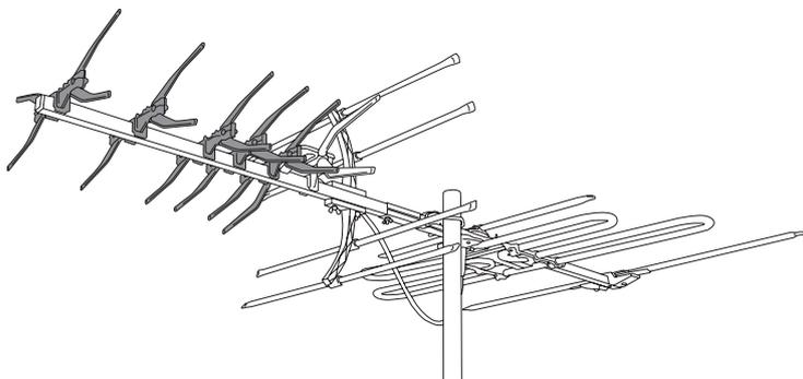
1) Snap on the five X type elements to the first five moulds located on the front 609mm boom.
