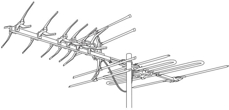
7) Connect the supplied 550mm interconnecting flylead by screwing one end onto the connection of the X type balun labelled "Input". Then, connect the other end to the G-units built-in balun. Finally, twist and push the rubber boots over the connections to create a weather seal.
