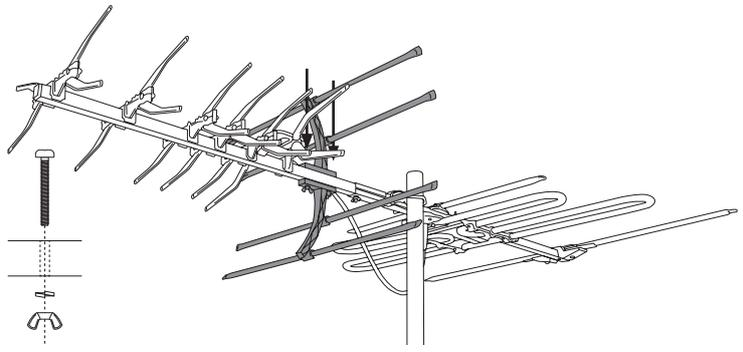
3) Install the two corner screens onto the top and underbody of the front 609mm boom behind the X type balun, using 3/16" x 1.75" Philips head bolts and two pre-drilled holes. Make sure you install the spring washer and wingnut on the underbody of the boom body.
