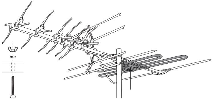
5) Attach the G-unit to the back 714mm boom underbody with the balun closer to the front of the antenna, lining up the pre-drilled holes located on the G-unit and boom. Bolt these two units together using the 1/4" bolt, flat washer, spring washer and wingnut provided in the small plastic bag. Ensure you install the flat washer, spring washer and wingnut on top of the boom body.
