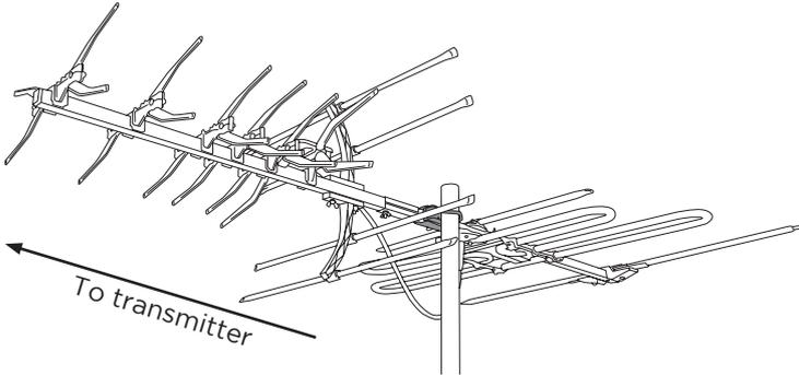
8) Attach the antenna to the mast using the U-bolt and point to your nearest transmitter. Slide the rubber boot seal into your coaxial cable. Strip the coaxial cable, attach the connector provided, and connect to the antennas X type balun labelled "Output". Fix the coaxial cable down the mast using UV grade insulation tape and cable ties.
