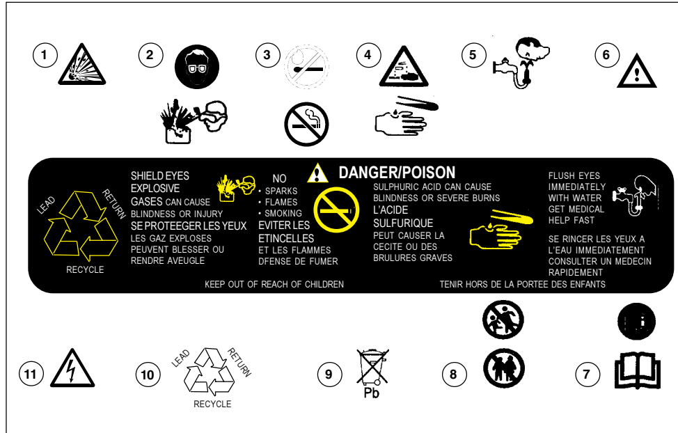
Fig. 1—Typical Battery Labelling
