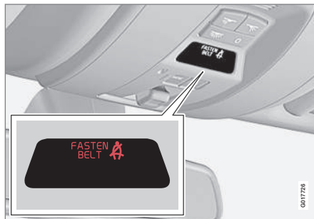
Seat belt reminder light in ceiling console
