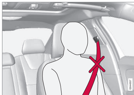
Incorrect height adjustment
