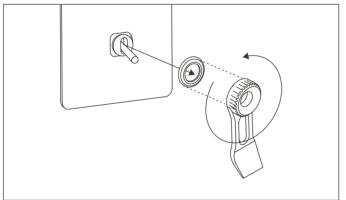
Toggle switches: use the remover tool to unscrew the toggle ring.
