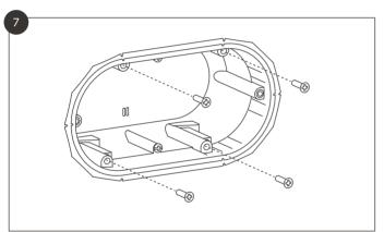
Plasterboard: push the box into the hole and screw in.
