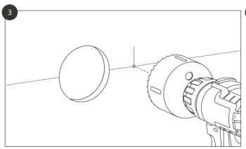
Using the markings as centrepoints, drill 71mm holes in the wall.
