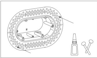
Brick wall: secure the box into the hole, for example with adhesive, or by nailing the trim down.
