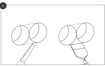
Remove excess wall between the holes.
