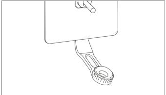
Slide the lip of the remover tool under the edge of the front plate and lever until it comes off.
