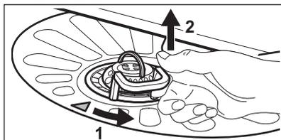
2. Remove the filter (C) out of filter (B).
