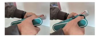
Step 1: Grab the magnetic seat of the pump with both hands and then rotate outward to open it
