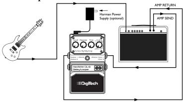
NOTE: if the amp effects loop has a mix control, set the mix to 100% full wet.
