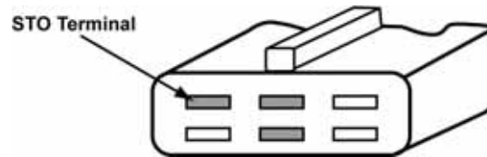
Figure 6-10 STO terminal on the 6-pin 4EAT test connector
