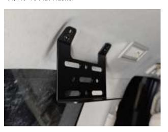
Assemble the cargo rack (E1&E2) and panel (D1&D2) and tighten the hardware.
