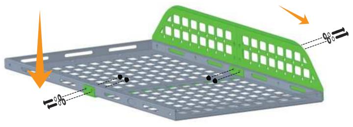
Step 5 Secure the cargo rack to the mounting bracket (A). Adjust it to the desired position. Finally, tighten all hardware. Repeat this step on the other side of the vehicle. •(4) M8×20 Button Bolt •(4) D8 Split Lock Washer •(4) M8×16 Flat Washer • (4) M8 Flange Lock Nut
