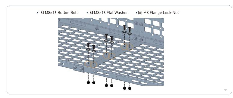
Secure the cargo rack to the mounting bracket (A). Adjust it to the desired position. Finally, tighten all hardware. Repeat this step on the other side of the vehicle.
