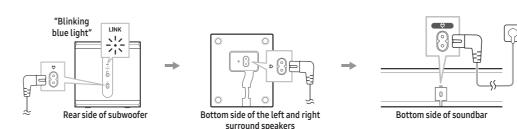
When the soundbar is properly connected to the subwoofer and surround speakers, the LINK LED indicator will stop blinking and turn solid
