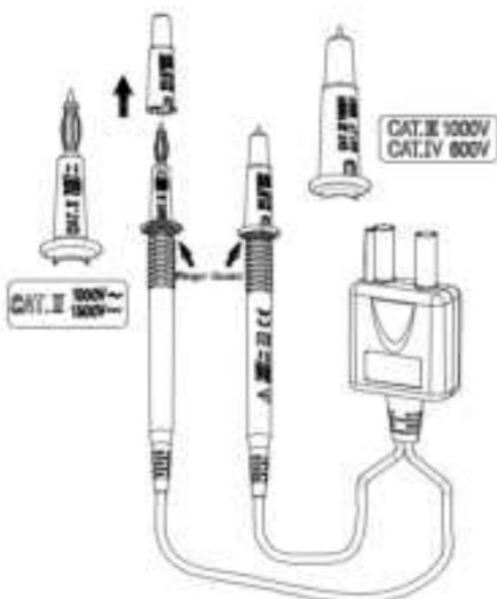
For CAT III or CAT IV environments, use the test leads with the probe tip guard cap fixed firmly. Without the probe tip guard cap, the test leads can be used in CAT II environment ONLY.
