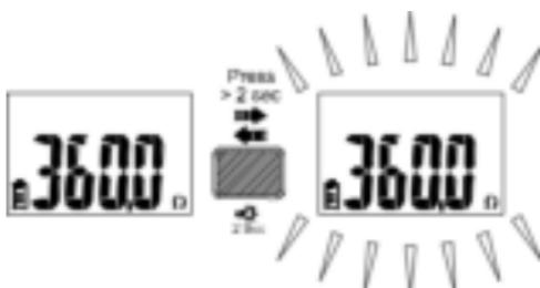
Press Function button for over 2 sec. to turn Backlight on / off.
