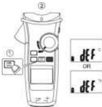
Turn on the meter after keeping MIN/MAX button down.
