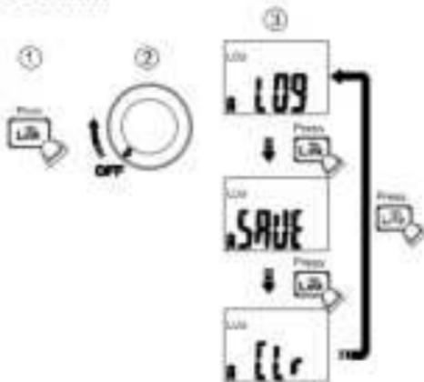
Pressing Link button while powering-up to select the mode – Logger mode, Manual Saving mode and Clear memory.
