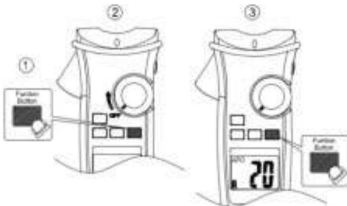
Press the function button and turn the meter on. Then press the function button to select the time. The time can be 5 minutes, 10 minutes, 20 minutes, and disabled (OFF).
