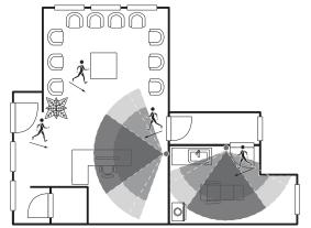
The examination room shows one Room Controller installed adjacent to the door. In this area of the room, occupant traffic is high and ensures the occupant will almost always cross the PIR detection path laterally and within the detection range.
