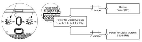
If a Relay Pack (or another isolated power supply) is used to power the Room Controller:
