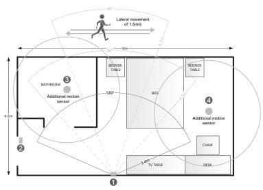
The internal Room Controller PIR sensor only detects lateral movement. It cannot detect movement when a person is moving toward it. It will not detect someone sitting on a chair and/or lying on the bed.
