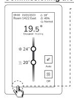
r - Tap and hold this area for 3 seconds to enter the set-up mode. When the list of users appears on the screen, tap to select the desired user, then enter the corresponding PIN code. This step is to prevent unauthorized access to the configuration menu parameters.
