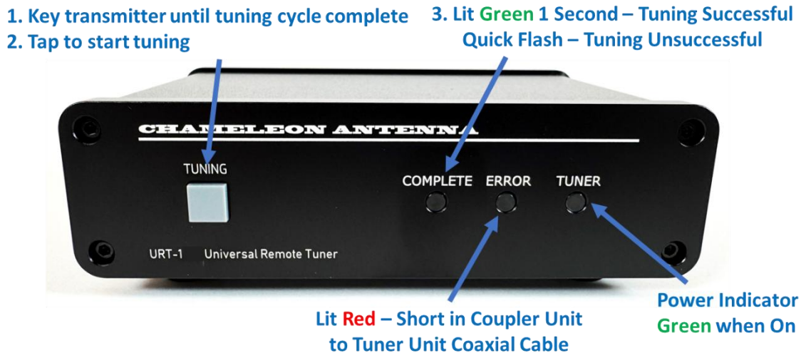
Figure 10. Coupler Unit Operation.
