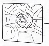
**3a.** Attach the rear wheel axle (G) to the chassis.
