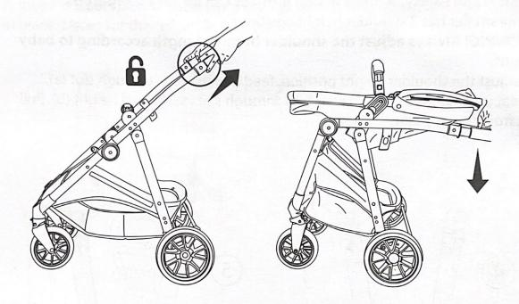
NOTE. The stroller cannot be folded in parent facing position.
