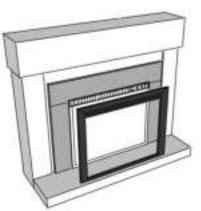
(5)Attach front face trim by hanging tabs on top, then pressing lower pins into spring clips at bottom
