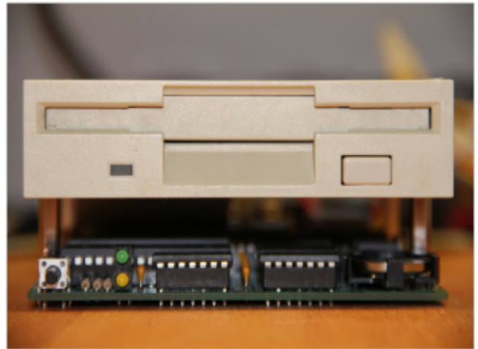
The 20Mhz Zeta board fitted underneath a 3.5" disk drive
