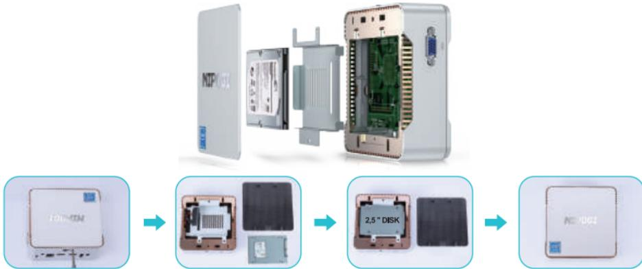
1. Remove one screw and then flipping a switch to take the cover off.
