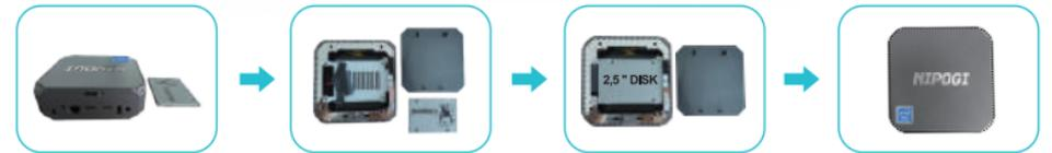
1. Move the switch/lever, there's a sliding "switch" on the top cover of the back that need to move over in order to remove the lid.
