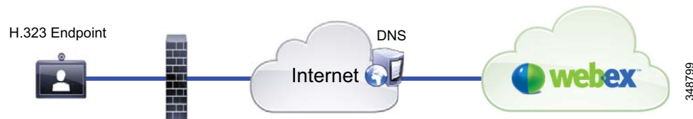
Figure 22-12 Cisco Collaboration Meeting Room Cloud Architecture Using H.323 Video Without Call Control System
