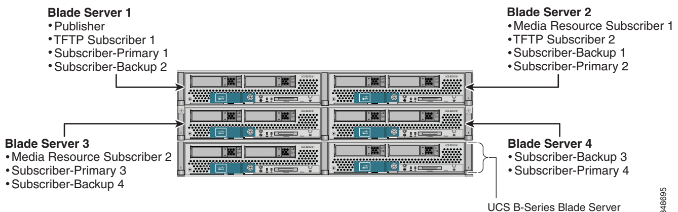
Figure 9-8 Unified CM Server Node Distribution on UCS
