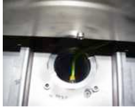
Earthing on the inside of the STF to a coupling screw
