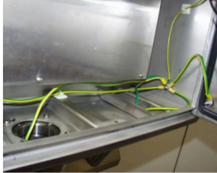
Earthing of the coupling to the housing (Similar to image)
