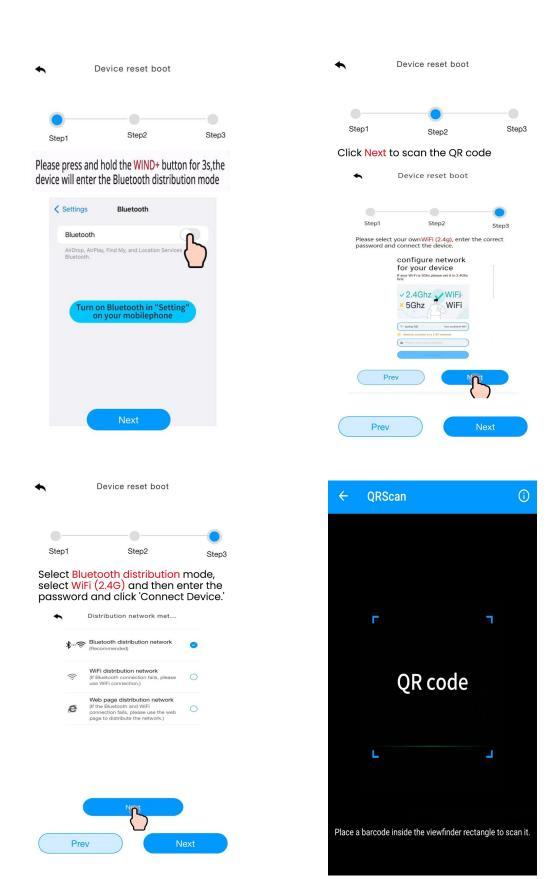
(4)Select the "WiFi Distribution Network" mode. Select your own WiFi (2.4g), enter the correct password and connect the device. After the connection is successful, return to the Device page.
