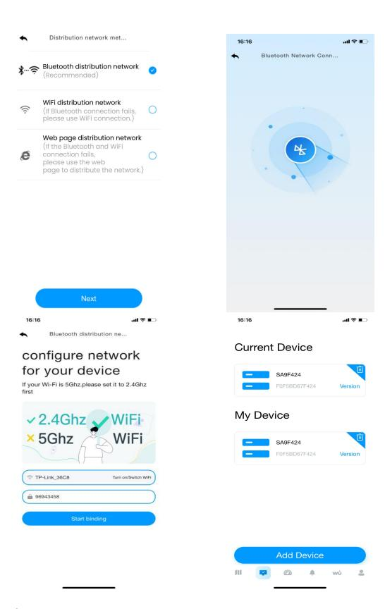
Note: If the connection via Bluetooth Distribution mode fails, please use the WiFi Distribution Network mode or Web Page Distribution Network mode to set up the network.
