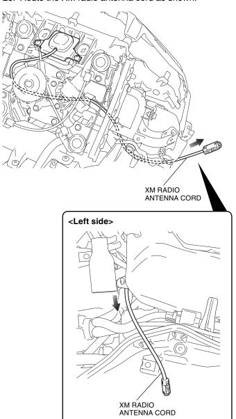
29. Route the XM radio sub cord as shown.Left side view, without top shelter for clarity>
