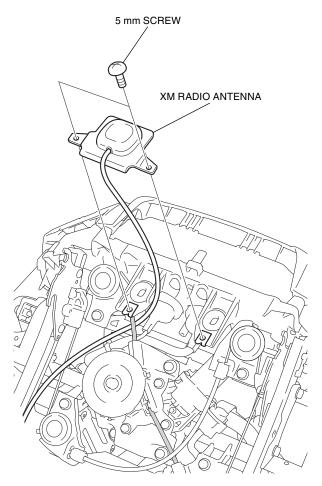
28. Route the XM radio antenna cord as shown.
