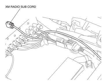
38. Connect the XM radio sub cord as shown.
