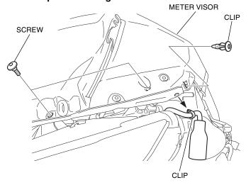
25. Remove the meter visor as shown.
