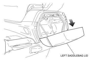
3. Remove the left side cover as shown, and disconnect the battery negative (-) cable.
