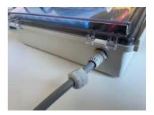
It is important to check the tightness of the cable gland before/at each use. If the cable is compressed, the nut may need to be retightened. It should not be possible to push the cable in or out with the correct pressure of the nut. A loose cable gland can cause water to get inside the battery box and damage and corrode the components inside.
