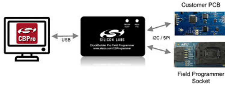
Figure 4.1. PC to CBPROG-DONGLE Connection
