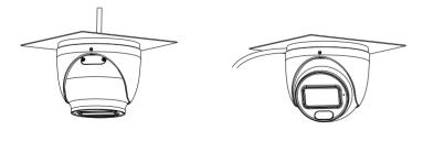
Then adjust the dome to obtain an optimum view angle.
