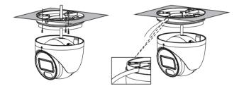
⑤ Install the dome and enclosure to the mounting base.
