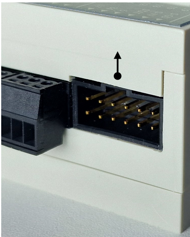
Figure 4: GPIO header location and pinout
