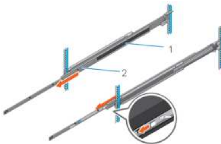
Figure 12. Pull out the intermediate rail
