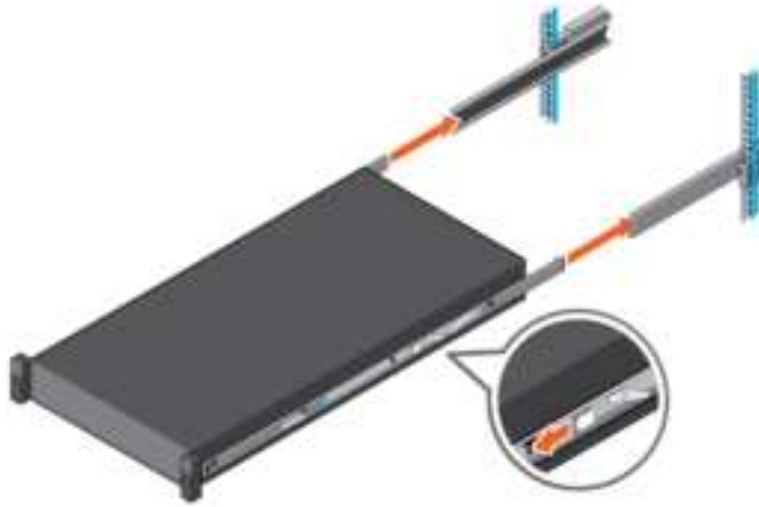
Figure 28. Install system into the extended rails
