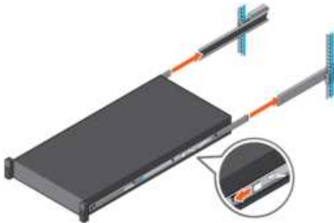
Figure 14. Install system into the extended rails
