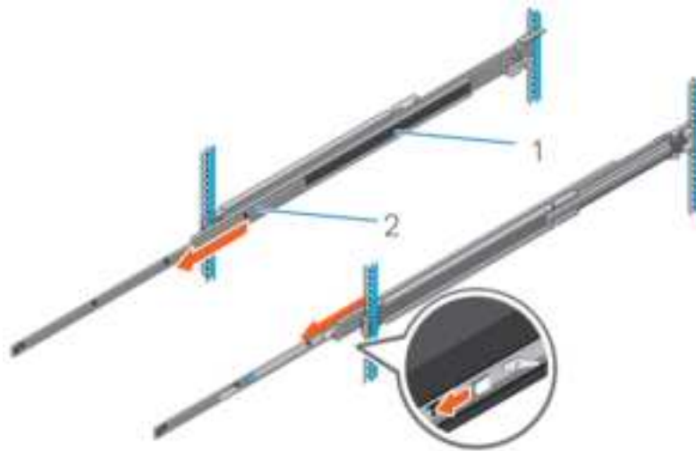
Figure 26. Pull out the intermediate rail
