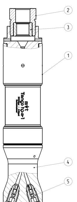
Important: identical-size nozzles must always be inserted diagonally opposite each other in order to prevent any imbalance occurring during rotation (risk of injury).
