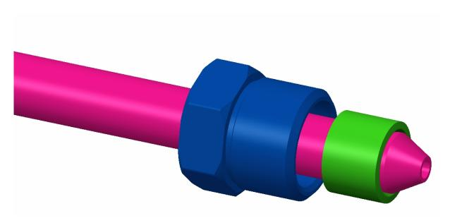
3. Insert the lance cone into the Tango nozzle's counter-cone.
