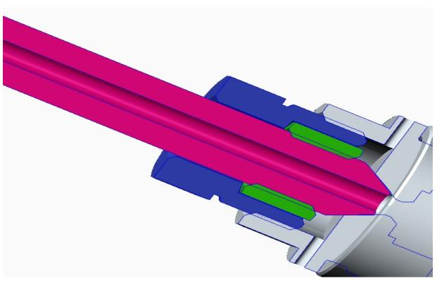
4. Screw in the M26 pressure screw and tighten it (tightening torque 70 Nm).
