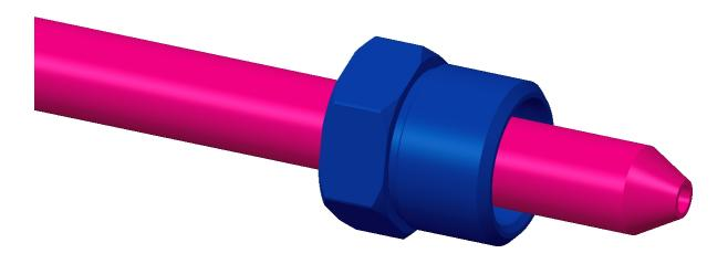
2. Screw the thrust ring onto the lance (left-hand thread). Screw the thrust ring onto the lance to the full extent of its threaded area.
