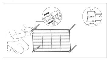
Please make sure that you have the Large Shelf(12) the correct way up. Hold the shelf on its side and slide it from the top of four lower poles down onto the plastic clips until there is a snug fit.
