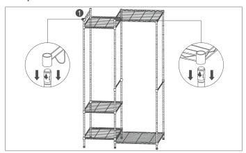
Refer step1 to snap the plastic clips(2) onto the same groove of the poles and assemble the last small shelf(5), and the last large shelf(12) at the the right of the top as well. Snap the plastic clips(2) on the two left poles and slide the support rail with hooks(1) on it.
