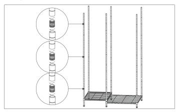
Screw the other poles on the assembled poles(Step3) by connectors(11). Repeat this step that four poles to build up one long pole.
