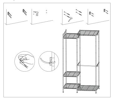
For the sake of safety, be sure to fasten the garment rack to the wall with the anti-tip devices included in the package.
