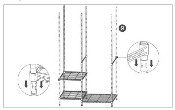
Snap the plastic clips(2) on the same groove of the poles which on the small shelf(5) and slide the second small shelf(5) from the top of the poles onto the plastic clips. Then snap the plastic clips(2) on the same groove of the poles which on the large shelf(12) and slide the support rail(9) on the plastic clips. These Shelf and Support rails can be adjustable randomly.
