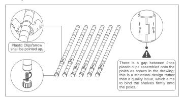
Screw the Leveling Feet(13) into the bottom of six poles. Then snap one pair of Plastic clips(2) on the groove of the lower pole (as the picture shows). Make sure the arrow of all plastic clips should be pointed up, and the groove of plastic clips should be locked with the poles.
