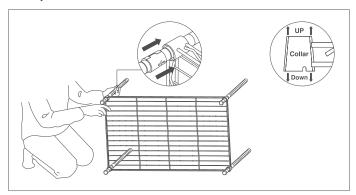
Please make sure that you have the Shelf way up correctly. Hold the shelf on its side and slide it from the top of four lower poles down onto the plastic clips until there is a snug fit.
