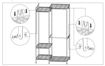
Assemble the Hook bracket(7) at the left and right of the Long clothes hanger rod(10) and the Short clothes hanger rod(3) by Screw(6). And hang the long hanger rod(10) under the top large shelf(12) and between the support rails(9), hang the short hanger rod(3) under the top small shelf(5).
