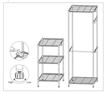
Pushing firmly down on every shelf at corners by rubber mallet to ensure all the shelves in a place over the plastic clips(2). Screw leveling feet(13) in or out to attain proper leveling. Now the clothing rack and shelf are already completely assembled.
