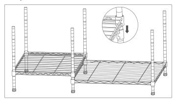
Refer to Step 1,2 to snap the plastic clips on the same groove of two poles on the large shelf(12) and assemble the small shelf(5). And then set the rack upright.
