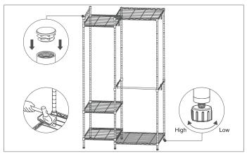
Put the plastic cap(6) on the top of the poles. Pushing firmly down on every shelf at corners by rubber mallet to ensure all the shelves in a place over the plastic clips(2). Screw leveling feet(13) in or out to attain proper leveling. Now the garment rack is already completely assembled.
