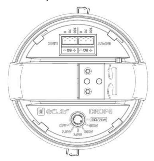
The DROP6 loudspeaker is delivered from the factory with the switch in the 60W position (70/100V). If accidentally connected to a low impedance amplifier (8 $\Omega$ ), it will not cause any damage to the loudspeaker, but it will under perform.
