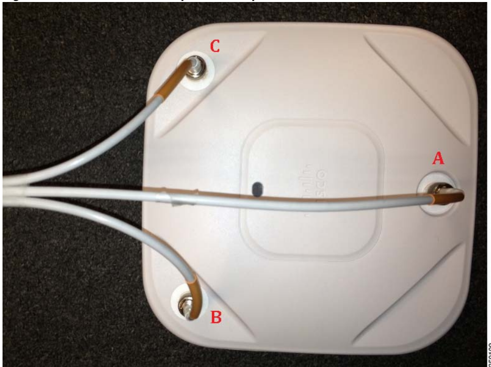
Figure 50 AP 1600 Note port “A” is Spaced Furthest from “B” and “C” for Best Diversity
