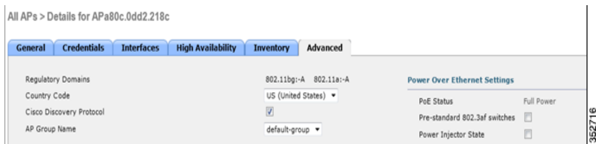
Figure 100 AUX port is active when PoE status is at FULL power or when a local power supply is used
