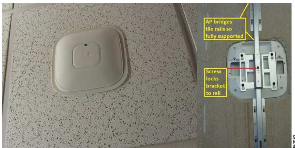
Figure 16 Optional AIR-AP-BRACKET-3 Used to Install the AP Directly Into the Tile
