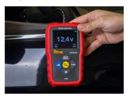
If the vehicle's battery voltage is correctly displayed upon connection of the PPDRAW, proceed to the next step.
