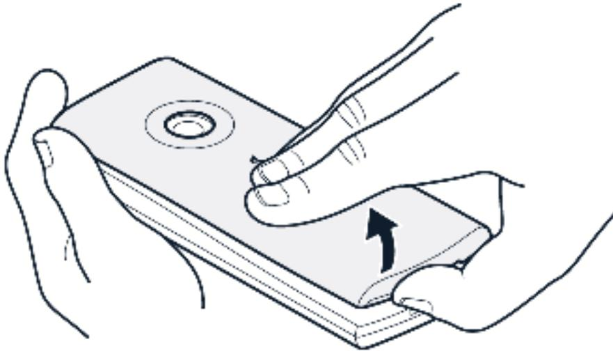
1. Place your fingernail in the small slot at the bottom of the phone, then lift and remove the cover.
