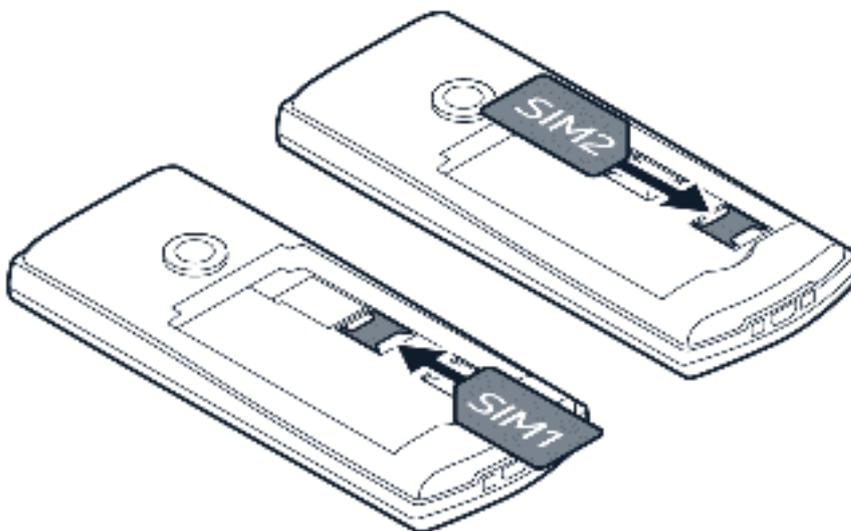
1. Slide the SIM card in the SIM card slot.
