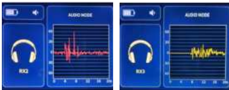
Figure : Characteristics of harmonic audio of false junctions such as semiconductors and metal-rusted junctions after tapping
